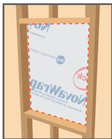
Cut around opening
